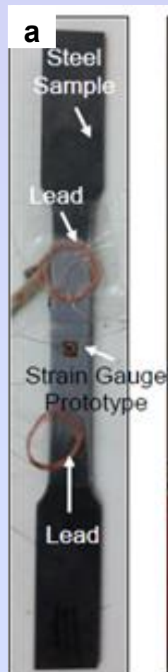
(a) Strain gauge consisting of CNT yarn in a metallic sample. (b) Strain and relative resistance change histories in five-cycle test with a 0.1%-maximum strain at a displacement rate of 1 mm/min. (c) Average gauge factor found for each displacement rate and pause length combination.
